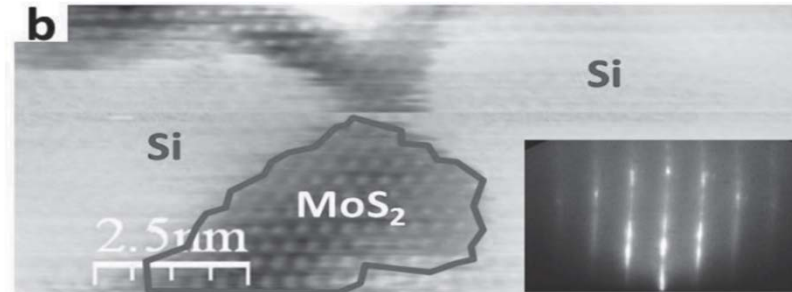
Fig. 4: Silicene on \text{MoS}_2 . Adv. Mater., 26, 2096-2101 (2014).
